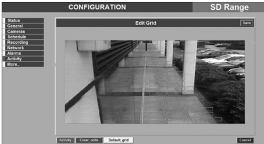
The alarm detection area can be edited via the Activity Grid. The Activity Grid can be used to exclude areas where there may be continuous movement (i.e. trees or bushes) which lead to false triggers. The camera view can be overlaid by a grid of up to 16x16 cells. Each cell can be individually enabled or disabled.
