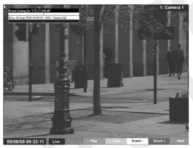
The screen displays the date, time and relevant server details for the event shown in the dialog box. A maximum of twenty events can be stored from connected devices. Use the Yellow and Green navigation buttons to move through the saved events.
