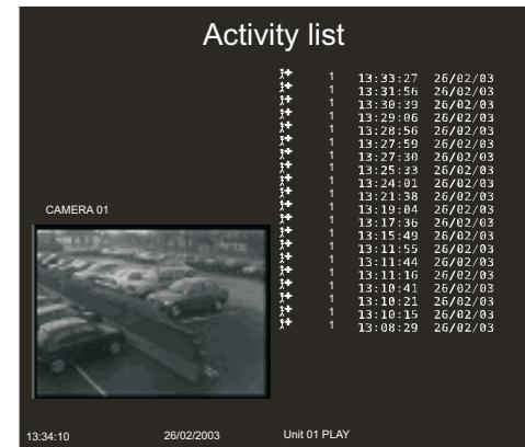
Use the **↑ ↓** keys to move the highlight up and down the list, the Activity image is automatically updated as the highlight moves. From this screen you can perform the following:
